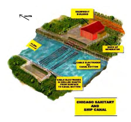
Figure 2: Plan view of how barrier electrodes are placed in canal bottom. (Source: <a href="http://images.suite101static.com/792724">http://images.suite101static.com/792724</a> com dbl.jpg (last accessed, October 7, 2010)
